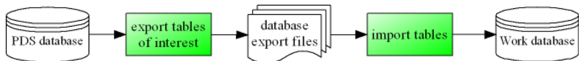
Figure 4-11: exporting the tables of interest from the PDS database to a separate database
