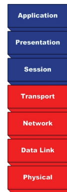
Figure 2.2: This figure shows the OSI model
