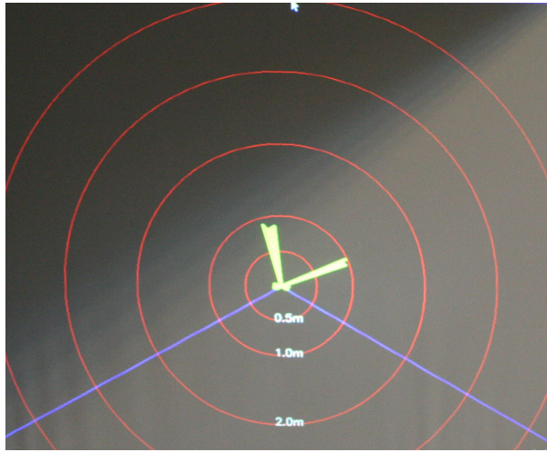
Figure 6.8: Example of lidar output. The outer edges of the green area denotes obstacles located approximately one meter away from the lidar. The blue lines are the view angle (240 degrees).
