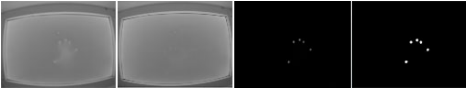
Figure 3.3: A series of images show how the image enhanced during the preprocessing. First image show the raw input from camera. Second image show the captured static background to be subtracted from the raw image. Third image show the subtracted image when a high pass filter has processed the image. Last image show the image after it has been amplified. The last image is the image fed to the tracking software.
