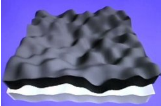
Figure A.4: Layers in Interpolating Force-Sensitive Resistance system. Image courtesy of www.touchco.com .
