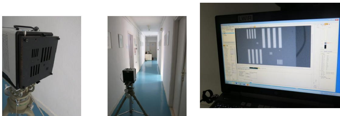
Figure 1. Set-up for MRTD measurement: left, black body with plate with slit patterns; middle, source and sensors; right, picture of PC screen during recording
