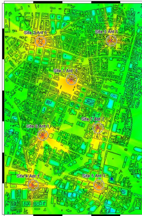
Figure 5.4: Map showing base station coverage in Dachau, Germany [Courtesy of Enorm GMBH].
