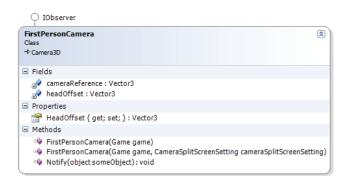
Figure 14.27: The FirstPersonCamera class.
