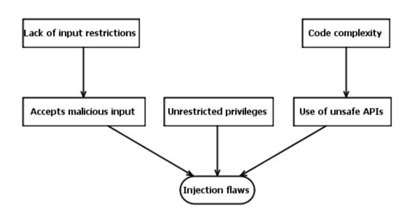
Figure 3.3: Vulnerability Cause Graph Example - Injection flaws
