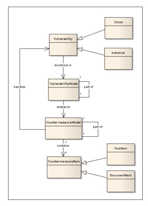
Figure 7.3: **Countermeasure Modelling Domain Model** - Concepts of countermeasure modelling (Use of this model is permitted by SINTEF)
