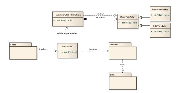
Figure 10.14: **High-Level Design with Security Pattern** - Intercepting Validator is instantiated
