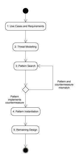
Figure 4.4: **Pattern Instantiation Workflow** - Pattern instantiation through design tools
