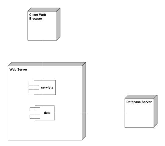
Figure 10.2: Case Deployment - The journal system is deployed on a Web server
