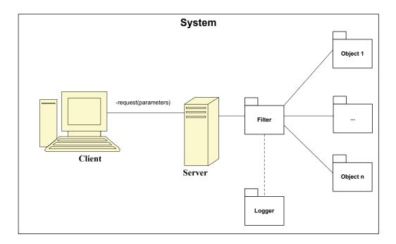
Figure 4.1: Client Input Filters - Pattern structure
