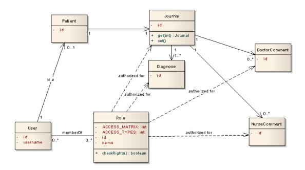
Figure 10.15: Data Layer Design with Security Pattern - RBAC is instantiated
