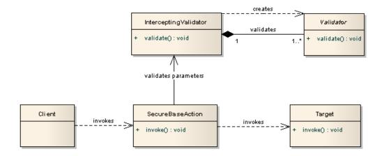
Figure 4.2: **Intercepting Validator** - Class diagram of the Intercepting Validator in Enterprise Architect.
