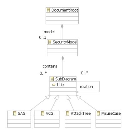
Figure 9.3: Extended SeaMonster Domain Model - SAG is added as a type of diagram
