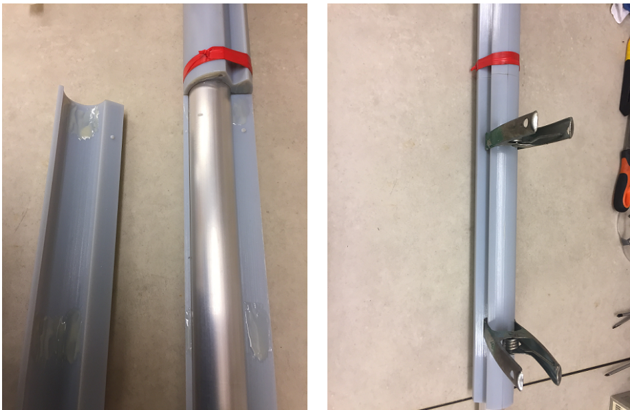
Figure 3.3: Gluing of 3D-printed parts to aluminum pipe.
