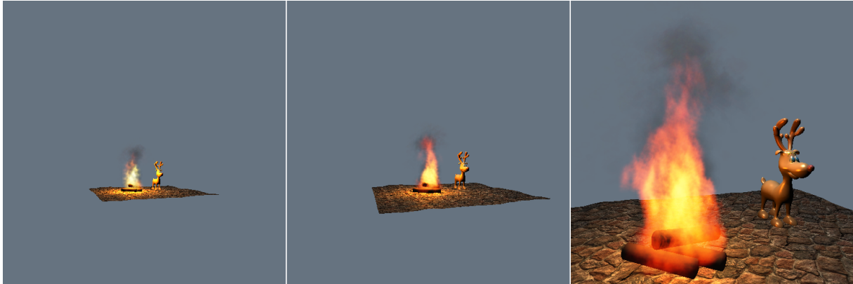
Figure 2: Screen captures from the third test. Fire rendering at different distances using 20, 200, and 4000 particles and simulation domain dimensions 16x24x16.
