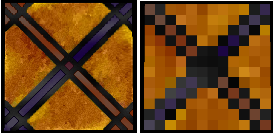
Figure 6.2: Single resized texture slice. Left: Slice is rendered as a full 128x128 texture. Right: Same texture after gradually using nearest neighbor filtering to scale it down to 12x12.
