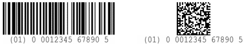
Figure 3.1: Information encoded using 1D and 2D barcodes
