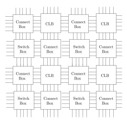
Figure 2.8: FPGA routing
