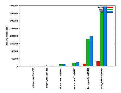
Figure 4.5: Different Memory Access patterns used by different configurations using the MemTest kernel.
