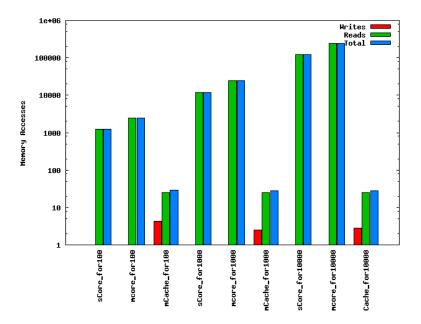
Figure 4.2: Different Memory Access patterns used by different configurations with the BogoMIPS kernel.
