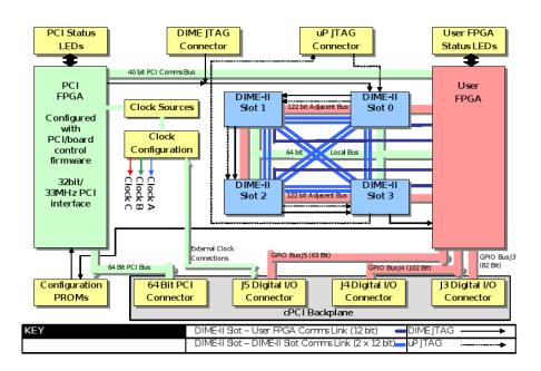
Figure 2.12: BenERA functional diagram [24]
