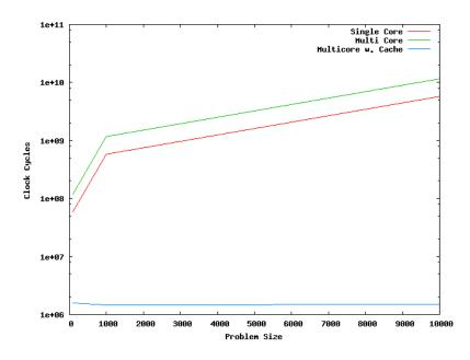
Figure 4.1: Different Configuration performance using the BogoMIPS kernel. Logarithmic Plot
