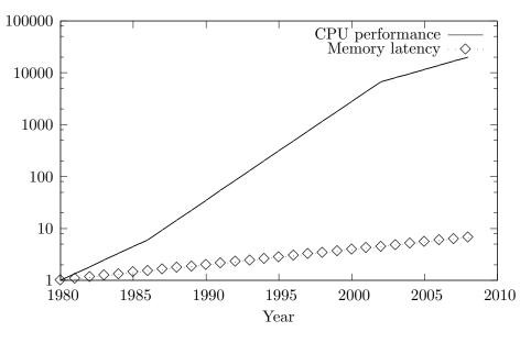
Figure 1.1: CPU/Memory performance[30]. Logarithmic plot for readability.
