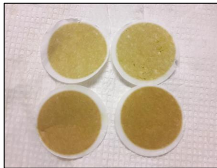
Fig. 6.5 POC filters after the seawater filtration
