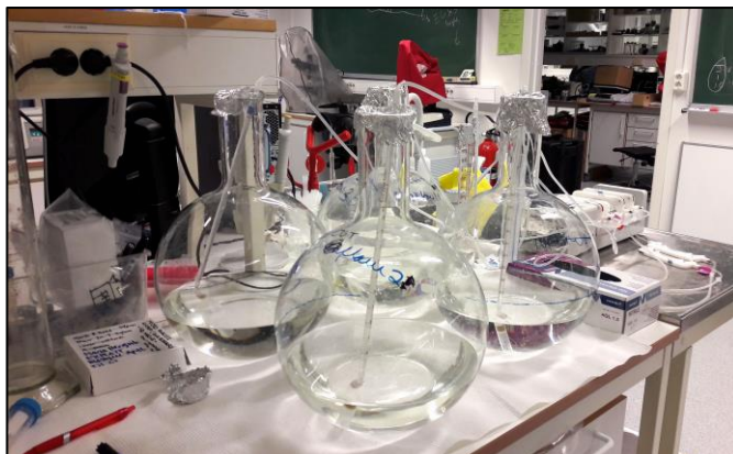
Fig. 6.6 Arrangement of solid phase extraction (SPE) Each PPL column was connected with a plastic tube joint to a pipette that was previously rinsed with methanol; the pipette was linked with a flexible plastic hose to a peristaltic pump. The PPL and glass pipette were placed inside the flat bottom flask. In order to ensure a full seal, Parafilm was used between the pipette and the flexible plastic tube.
