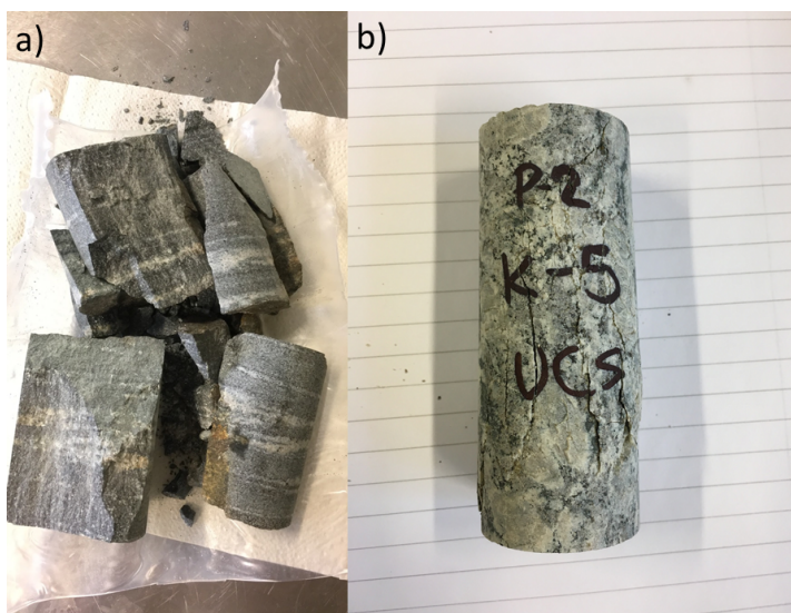
Figure 3.9: The behavior of sample 1 and sample 2 was different, both prior to and during failure. a) Sample 1 broke into several small pieces with no clear rupture angle.; b) Sample 2 behaved like a typical granite, and the fracture angle could be determined from some of the cores.
