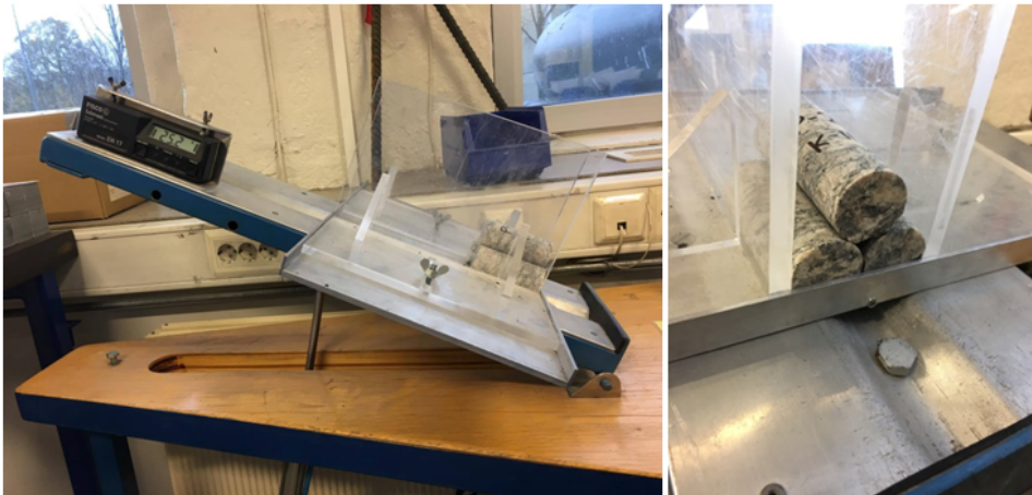
Figure 3.12: The basic principles of the three core tilt test following the standards from Li et al. (2017). The core was lifted at a constant speed until the upper core started sliding.
