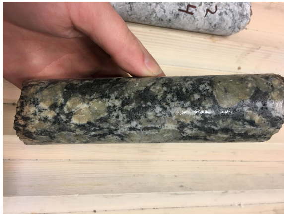
Figure 5.7: Sample of the porphyritic granite with several large feldspar crystals present in the sample.
