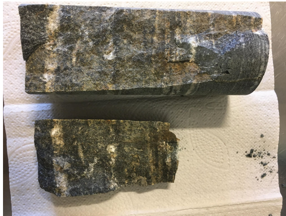
Figure 5.6: Granitic gneiss with failure located along a weakness zone in the core. The measurements for this sample were not included in the calculation of the rock mass parameters
