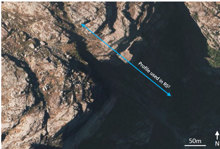
Figure 3.17: Illustration of the position of the profile exported from ArcMap to RS 2 . The profile was based on the high quality point cloud obtained from the drone model.
