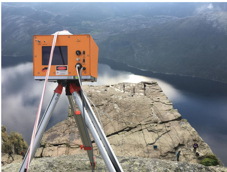
Figure 3.3: The Optech ILRIS-3D LR during the closes scan (scan 3) with a mean distance of 40 m.
