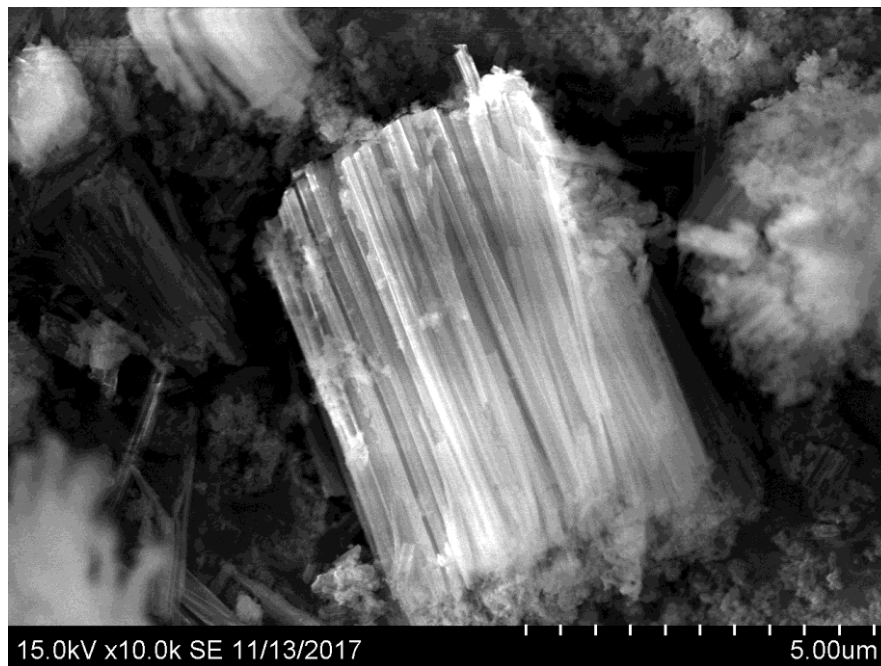
Figure 4.20. When scratching of the nanostructure as a powder, it can be observed bundles of nanowires. This image has a 10k magnification.
