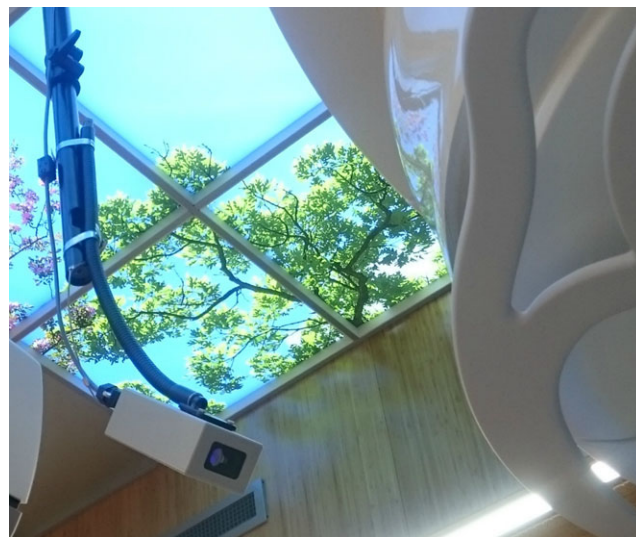
Fig. 1. Laser measurer mounted on the ceiling in the treatment room.
