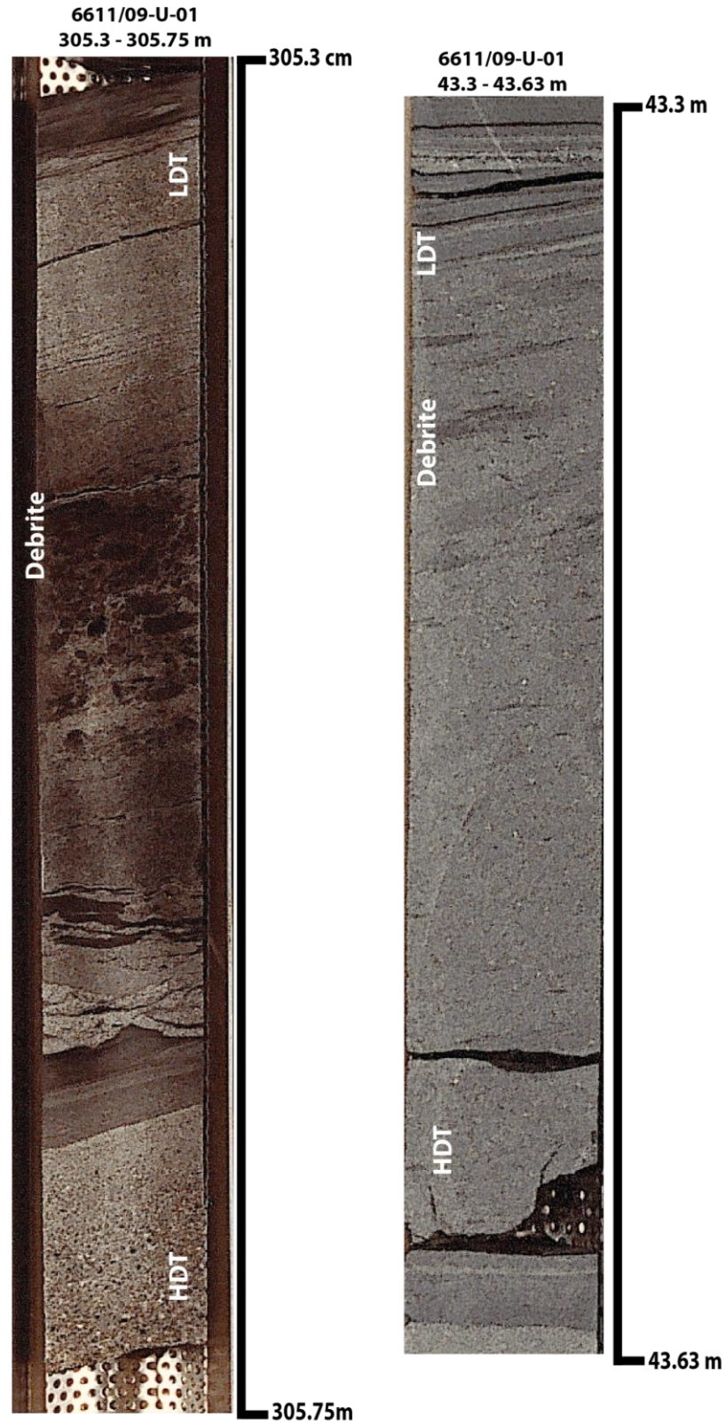
Fig. 44: Core photos showing facies association of debrite underlain by massive sandstone (high density turbidite/HDT) and overlain by low density turbidite (LDT)
