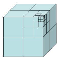
Figure 4.3: Multi-resolution. The nearest, upper subvolume is expanded 3 levels
