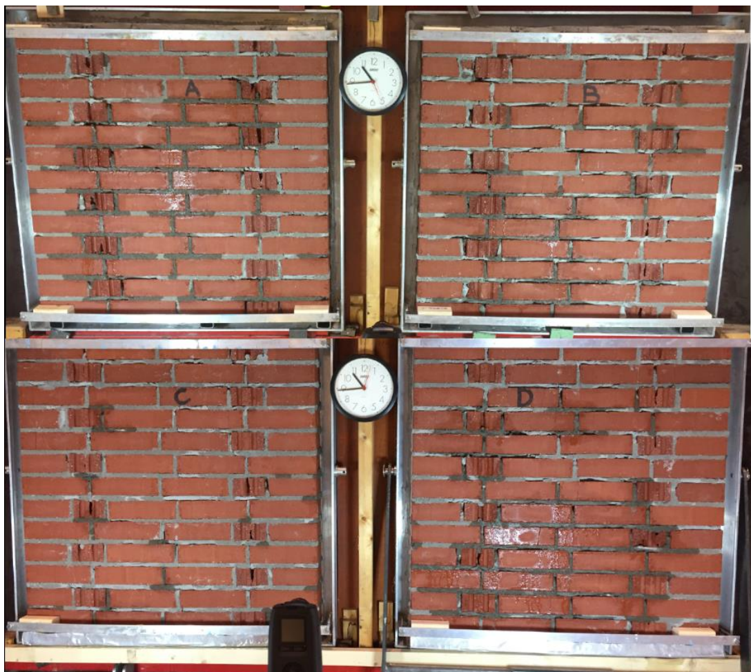
Figure 4. Panels A, B, C and D after 45 minutes of simulated driving rain.
