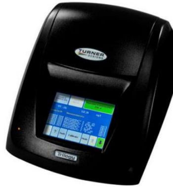
Figure 4-3 Fluorometer - Turner Designs. Chlorophyll a content of the cells was measured by Trilogi® Laboratory. (Designs, 2017)
