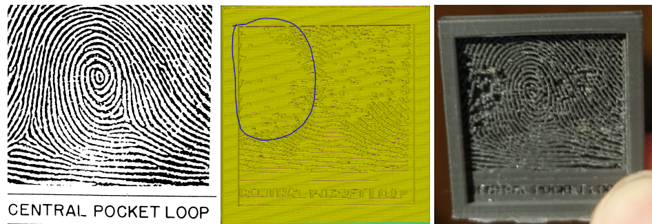
Figure 11: A left B middle C right - First attempts making model from [4], with error propagation seen in image C).
