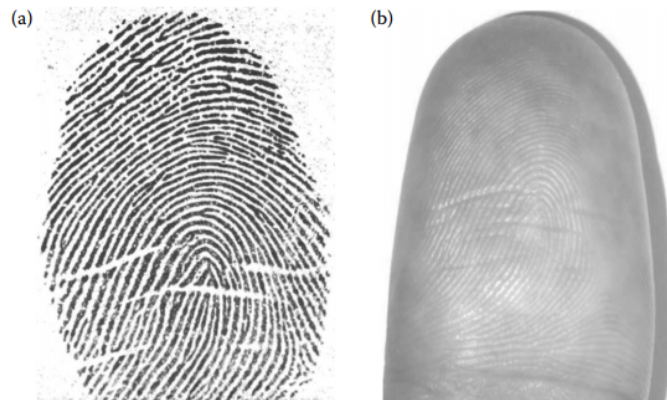
Figure 3: Showing captures from a traditional optical sensor(a) and a touch less optical sensor(b)[5]
