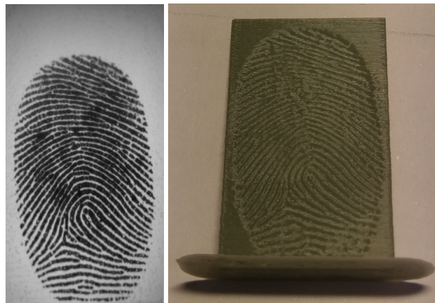
Figure 26: Source picture from FVC2002(40_1), and artefact generated using PLA 1.75mm thread
