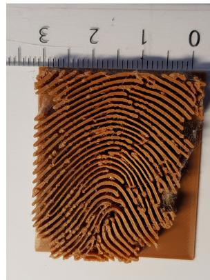
Figure 18: PLA 1.755 filling, ignoring thickness
