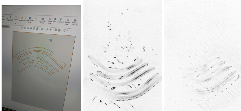
Figure 35: a) model used for generating artefact. b) artefact on sensor with a depth of 0.5mm c) flexible filament fused with conductive filament with a thickness of 0.3mm
