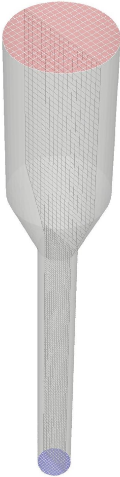
Figure 90 - The geometry with the 2 cm mesh used in this study. The inlet is indicated in blue and the outlet in red.
