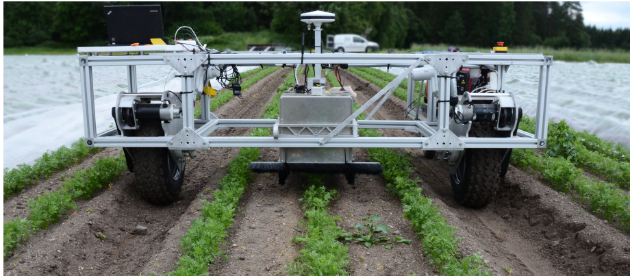
Figure 16: Asterix prototype gathering data from a carrot field (Rygge 2014).
