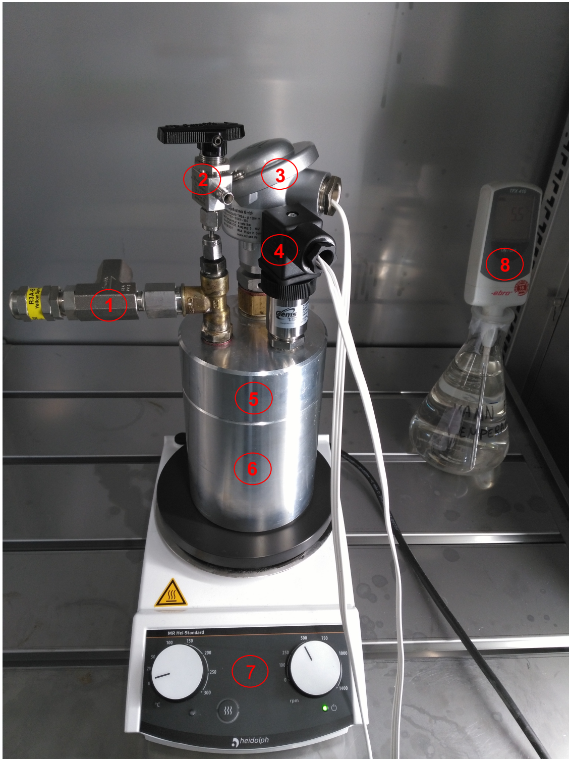
Figure 3.1: Picture of the experimental apparatus inside the refrigerator. The various components present inside the refrigerator when running the experiment are numbered from one to eight. 1: Relief valve, 2: 3-way-valve, 3: Temperature sensor, 4: Pressure sensor, 5: Steel cap, 6: Steel cylinder, 7: Magnetic stirrer, 8: External temperature sensor placed in water filled Erlenmeyer flask (Helgestad, B., 2017)
