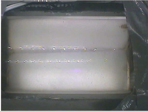
(a) There is no hydrates observed through the sapphire optical section at this stage in the experiment (time: 13:05).
