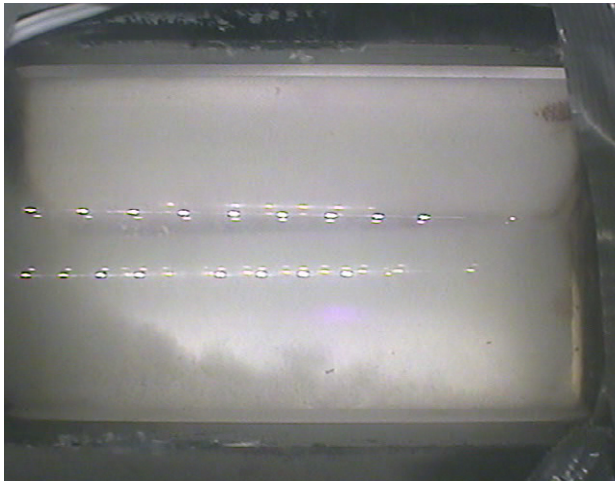
(c) Hydrate slurry observed in the lower, left corner (darker area) through the sapphire optical section in the wheel 15:16.
