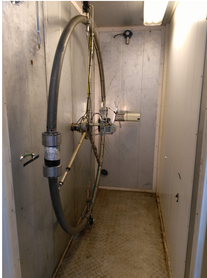
Figure 3.5: Picture of the Wheel Flow Loop inside the climate chamber (Helgestad, B., 2017) .
