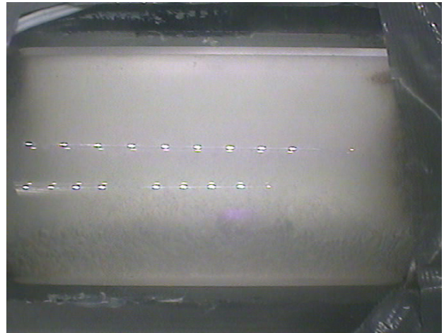
(d) A hydrates slurry is observed along the lower part through the sapphire optical section in the wheel (time: 15:18).
