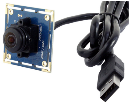
Figure 2.4: Fish-eye camera inside ROV uDrone (Source: Henriksen & Sandøy (2015) ).
