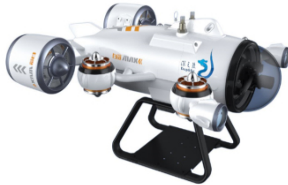
Figure 1.1: DeepFar MAX ROV (Source: deepinfar.com).
