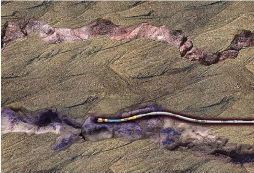
Figure 2-6: Artistic illustration of a high local dogleg developed at the surface of a calcite cemented stringer (Hood et al. 2003).
