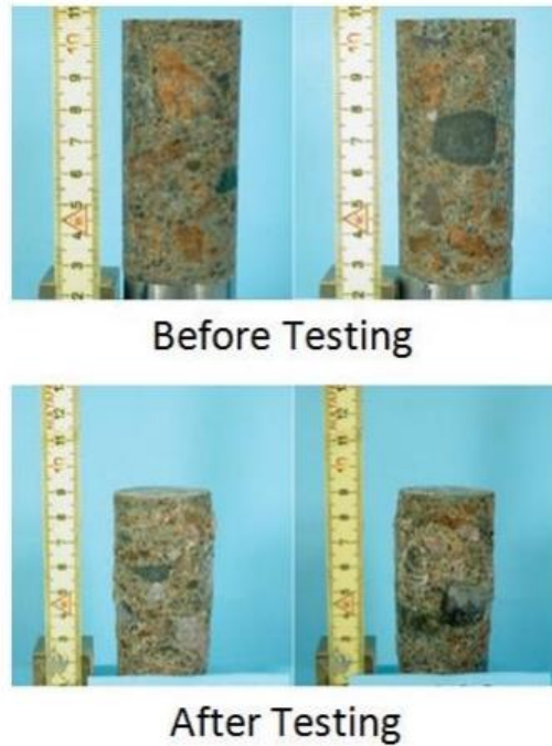
Figure 3-4: Triaxial test sample from weak matrix conglomerate from the Edvard Grieg field (Hilgedick et al. 2012)
