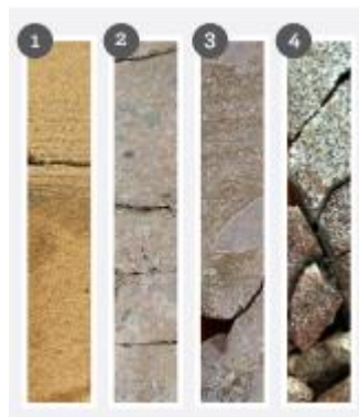
Figure 3-1: The four different reservoir types of the Edvard Grieg field. 1- Sandstone, 2- Conglomeratic sandstone, 3- Conglomerate, 4- Weathered and fractured basement (LundinNorwayAS 2014).
