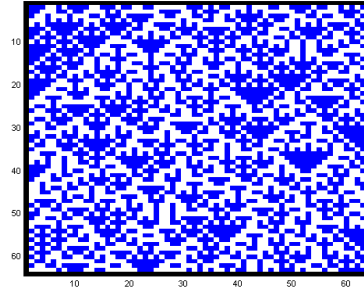
Fig. 4. Target generated using a cellular-automata with rule 90 of Wolfram starting from a random initial line (64x64).
