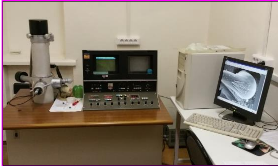
Figure 3: Scanning Electron Micrograph, HITACHI S405-A, at the White Sea Biological Station (Photo: Tuva Bongard Munkeby).
