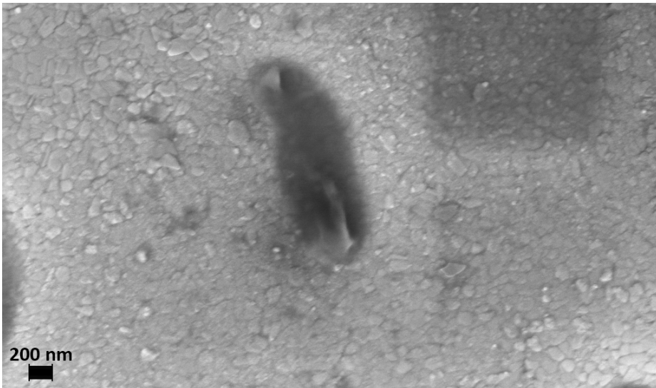
Figure D.5: SEM image showing the microstructure of the KNN25 thin film after being soaked for 14 days.
