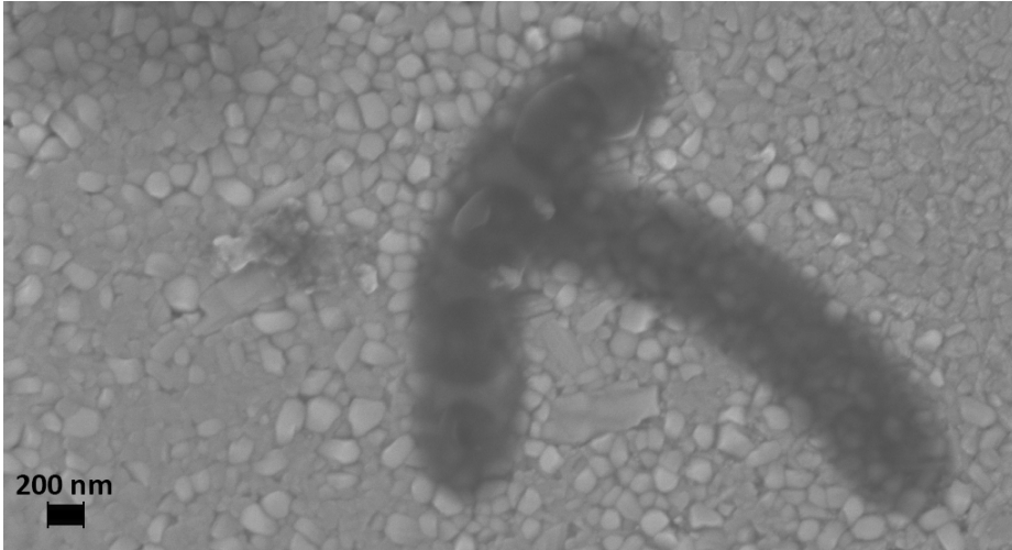
Figure D.4: SEM image showing the microstructure of the KNN25 thin film after being soaked for 10 days.
