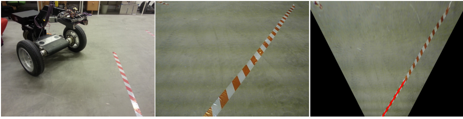
FIGURE 7.2: Test with Dogmatix to ensure the mapping of an identified line is accurate. Robot pose is (x, y, \psi) \approx (0, -1.0, \pi/4) . The left picture shows the robot's orientation to the line, the middle image shows the raw camera input, and the right image shows the input after projective transformation with the identified line found using least squares method.
