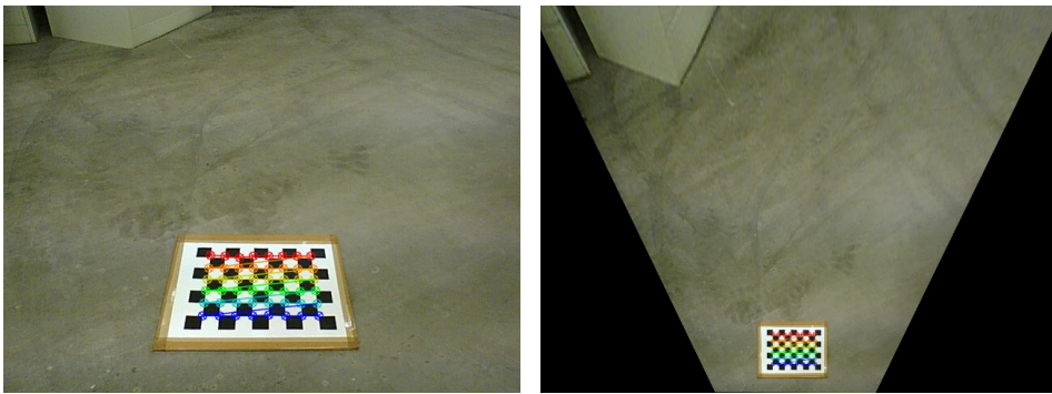
FIGURE 5.8: The left image shows a picture of a chessboard pattern taken with the camera mounted on Dogmatix. All identified corners have been marked with circles and lines and are used to find a homography matrix for a projective transform. The right image shows the same picture after the projective transformation.
