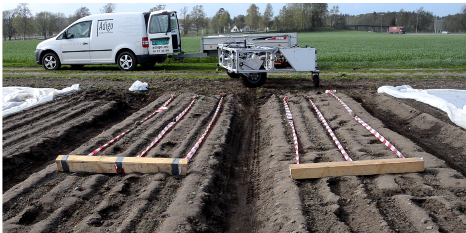
FIGURE 8.4: A test of the identification and turning strategy at the end of a row. The robot successfully identified the end, kept driving straight for a specified length to completely exit the row, turned around, identified next row and continued with following it.
