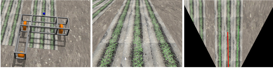
FIGURE 6.5: Simulation of row detection, estimation and following. The robot starts in the position shown in the left image and attempts to follow the middle row. The middle image is the raw camera input, and the right image is the projected image with identified lines.
