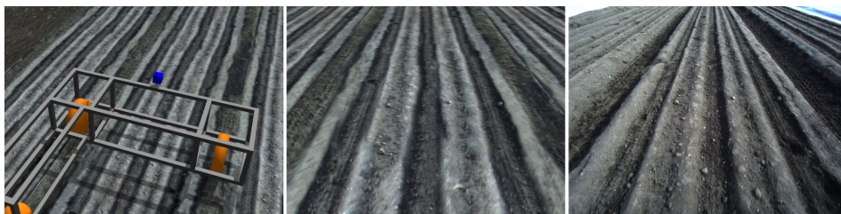
FIGURE 8.5: Left image shows the simulated robot placed in the simulated field, middle image is captured by the simulated robot, and right image is a real picture captured by Asterix.
