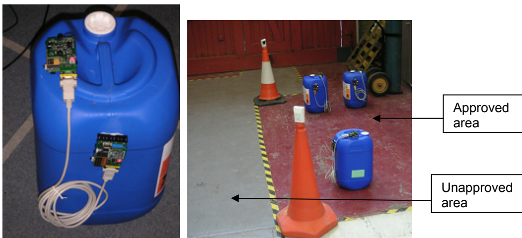
Figure 23: Left: physical view of an intelligent chemicals container. Right: Intelligent Container Test Bed
