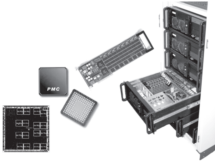
Figure 1. A MISD processor die containing 1024 parallel elements are packaged and mounted in quantities of 16 chips on a PCI accelerator card. Multiple cards are inserted into a PC node, which servers as the building block for the cluster.
