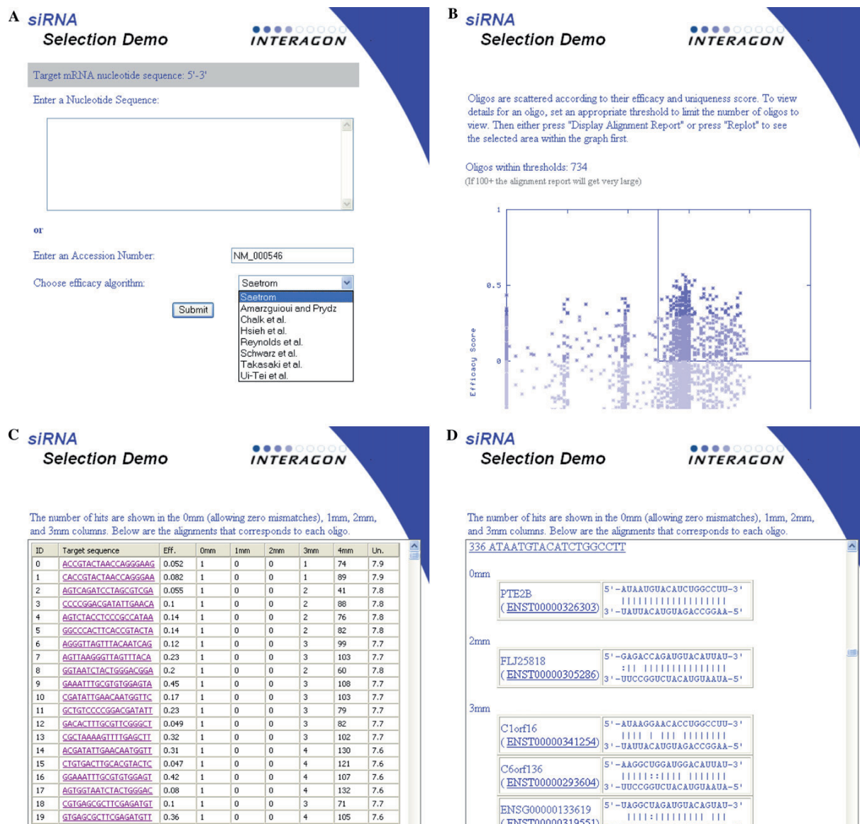
Fig. 1. Screenshots of (A) the selection screen where the users input the RNA sequence or accession number and choose an siRNA efficacy predictor; (B) the scatter plot showing predicted efficacy versus uniqueness for each siRNA; (C) the result overview where the siRNAs are ranked according to predicted efficacy and uniqueness; and (D) the alignment of the ranked siRNAs with potential off-target regions.
