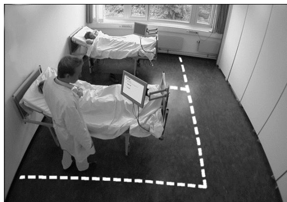
Fig. 3: User location / fixed device: The fixed bedside terminal responds as the hospital worker enters the virtual zone, and presents the associated electronic medication chart.
