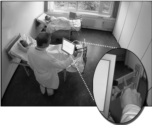
Fig. 5. Mobile token / fixed device: Scanning a mobile barcode card with the reader attached to the fixed display retrieves the electronic medication chart.
