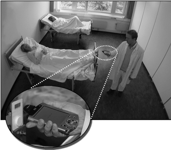
Fig. 4. Fixed token / mobile device: A patient's electronic medication chart is retrieved by scanning the fixed token attached to his or her bed.
