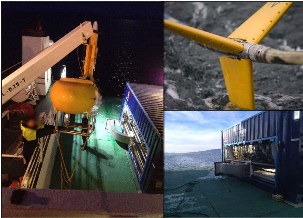
Figure 10.1: Field test. Tail-buoy in left photo (mounted on the aft of the cable), the Bird mounted on the cable in the up-right photo and the seismic cable winch in the down-right photo.
