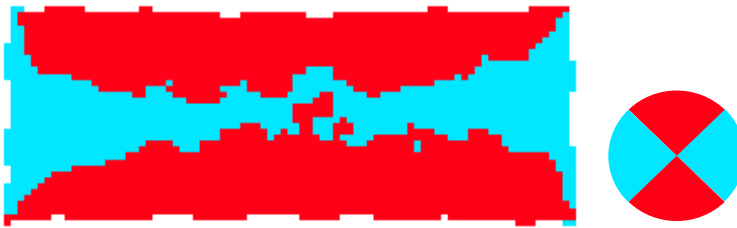
Figure 4.10: Retrieving the orientation distribution from experimental data assuming 2 possible orientations. The value of the cost term was set high to emphasise how it controls the simulation. The retrieval was done over 56 annealing cycles with 1000 Monte-Carlo steps per cycle.
