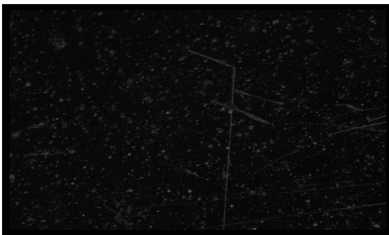
Figure 8.4: Dark-field image built up of 24 images with NA_{illu} > NA_{lens} and 1 LED lit each.
