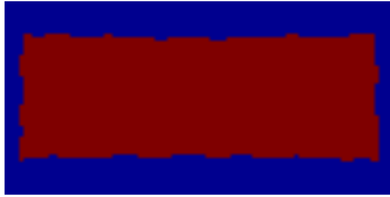
Figure 3.7: Image of the theoretical sample used for retrieving the orientation distribution. The red area is the sample, and the blue is air padding added around. It does not look like a smooth shape since this sample used only used 1/16 of the regions of the theoretical sample that was made. It consisted of 2851 regions, also called voxels.
