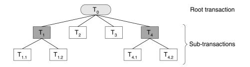
*Figure 4.1 Illustration of the nested transaction model.*
