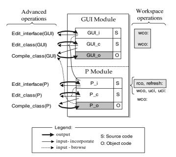
Figure 7.13 Illustration of workspace operations applied on GUI and P modules.
