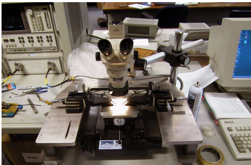
Figure 4.25. Probe station and the measurement setup.
