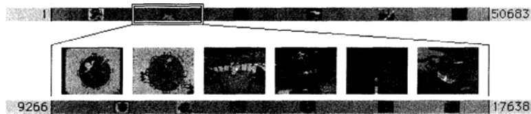
Figure 3.34: Hierarchical Video Magnifier, one level (adapted from [Mills et al. 1992])
