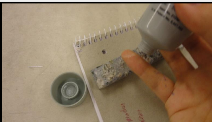
5) Add a dab of vacuum grease to your finger.
