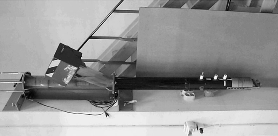
Figure 4.4: The circular Kundt's tube used for the impedance measurements. Note that the figure has been rotated counterclockwise. The samples and the reflecting end piece are mounted from below and are held in place by the "clamp" at the bottom. There is no visual control of the mounted samples.
