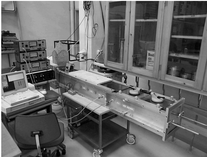
Figure 3.6: The Kundt's tube, with microphone amplifiers to the left. Two of the tube walls, and also the movable "piston" which constitute the back wall, are made of glass. This allows for visual control of the mounted sample, and also vibration measurements by laser interferometry, as described in Ch. 4. In the background can be seen the anechoic end piece used during the calibration.
