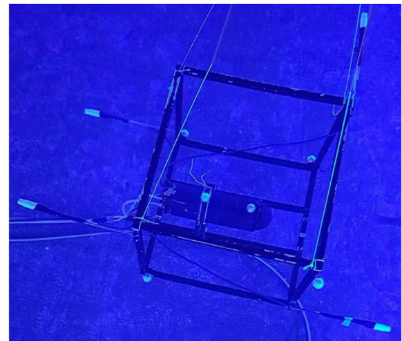
Fig. 5. The sensor platform with hydroacoustic transducers (on rods), Qualisys markers (reflective balls), and an underwater housing. The blue light is emitted from the OQUS camera system in order to better detect the reflective markers. (For interpretation of the references to color in this figure legend, the reader is referred to the Web version of this article.)
