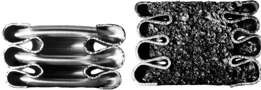
Figure 6 Axial crushing of non-filled and foam-filled circular and square extrusions, quasi-static loading
