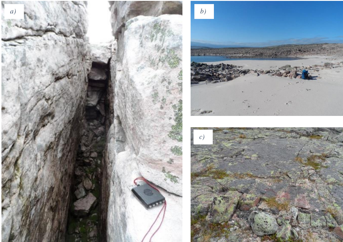
Figure 5.23: a) Weathering along open joint in Unit B, fracture planes have a sugary texture extending outwards. b) Image from the top of the Vaggecearru Mountain, where unconsolidated sand covers the bedrock. c) Closed joints in Unit C.
