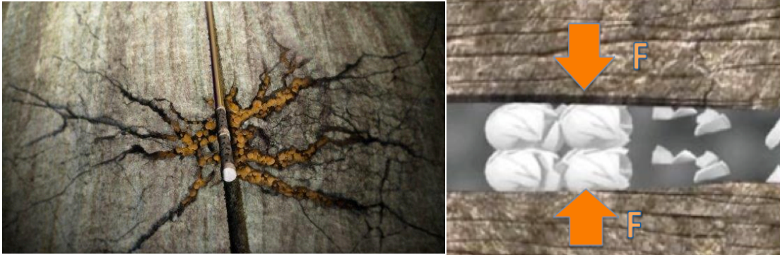
Figure 3.1: Illustration of proppants deployed in a fractured reservoir, and fines generation introduced by crushing of proppant under high closures stress ( F ).
