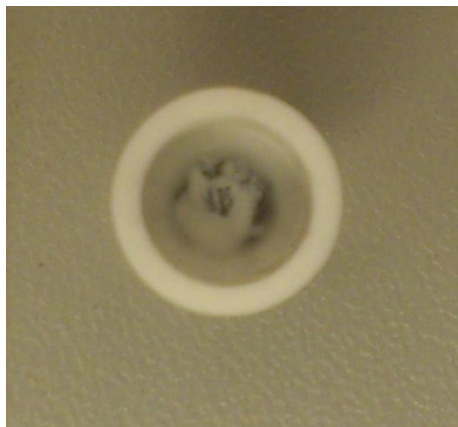
Figure 4.6: Top view of wool-like formations on the surface and upwards (i.e. only the grains at the very top was clad in this wool-like formation) of the sample. This picture is the same illustrated in Figure 4.5.middle, sample coarse C.
