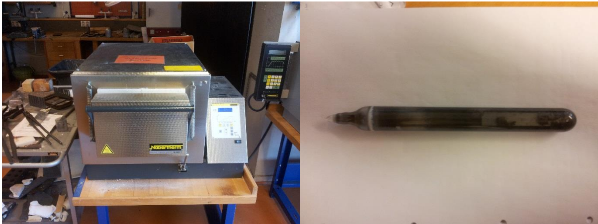
Figure 22: Left : Nabertherm N17/HR was used as furnace for the second heat treatment. Right : The ampoules (after solution annealing and aging) used to seal off the material from the environment in the furnace
