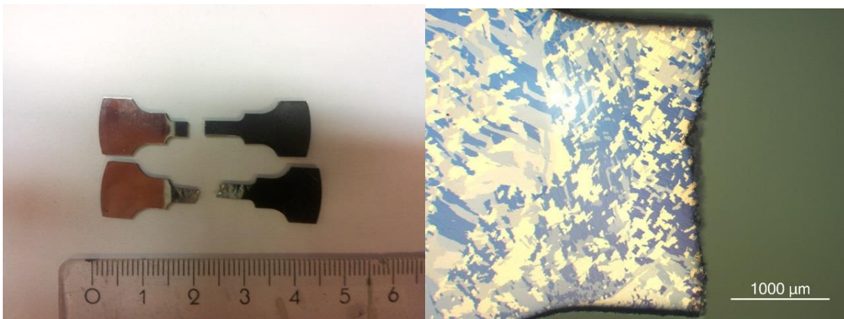
Figure 48: Left: The tensile specimen at the top is contaminated, while the tensile specimen at the bottom is the as-received material. The contaminated specimen fractured around 300 MPa, while the bottom specimen fracture around 10% elongation. Right: Tensile specimen (AC) observed in Leica MEF4M with polarized light. The sample went to fracture before the tensile test could start, i.e. during clamping/fastening.
