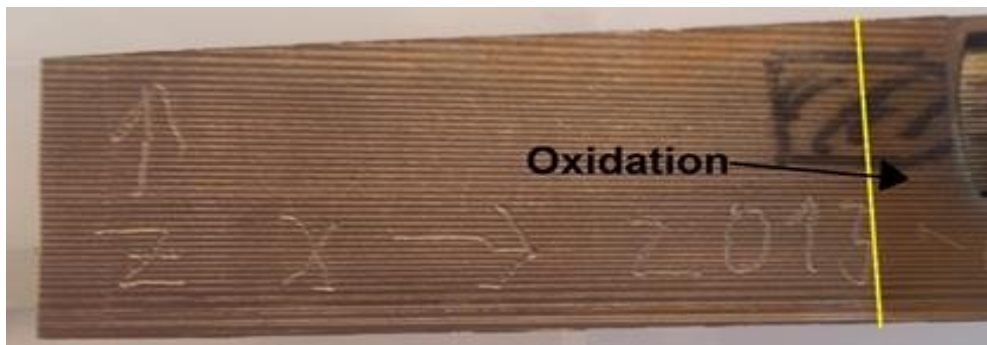
Figure 47: Showing the oxidation present on the material after spark cutting. The oxidation is observed as a brown/darker surface than the original material.
