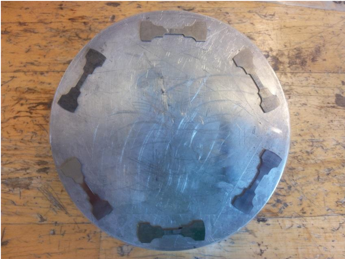
Figure 19: Showing a typical mounting of the tensile bars on the sample holder. The samples are oriented in the circumference direction, and is evenly distributed around the circumference to have the loading as even as possible on each sample.
