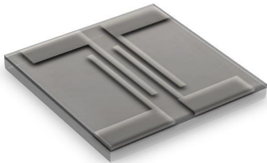
Figure 16. Illustration of a glass slide after completing the metal deposition-step of the manufacturing procedure.
