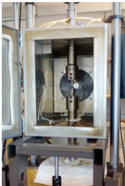
Figure 3.3 – MTS 880 tensile testing machine equipped with a furnace chamber positioned around the specimen.
