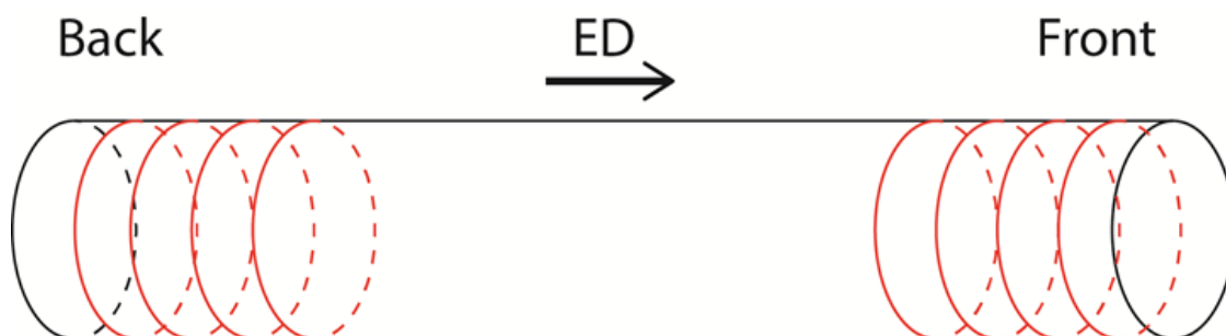
Figure 21: Schematic illustration of the collection of samples for artificial aging.
