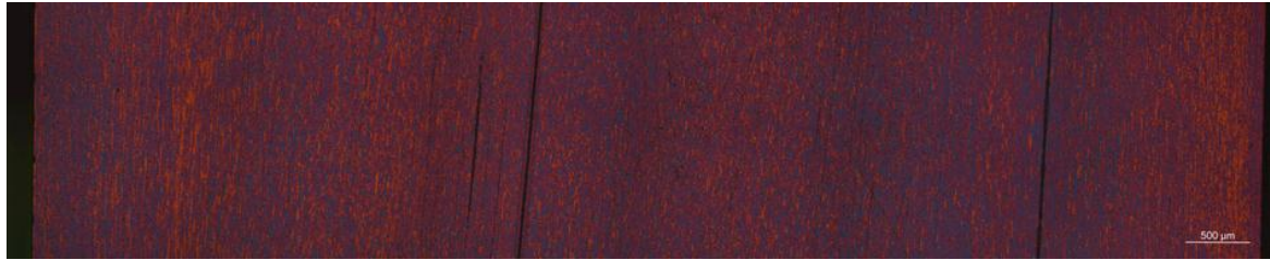
Figure 55: OM of RSA6061 T6 540, measuring bar is 500μm, SSHT at 540°C.
