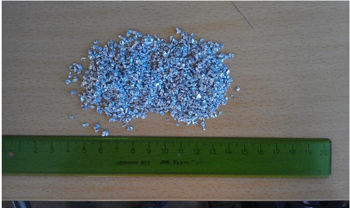
Figure 16: Representative collection of the granulates (cut from ribbons) obtained from RSP-Technology, Alloy RSP6061.
