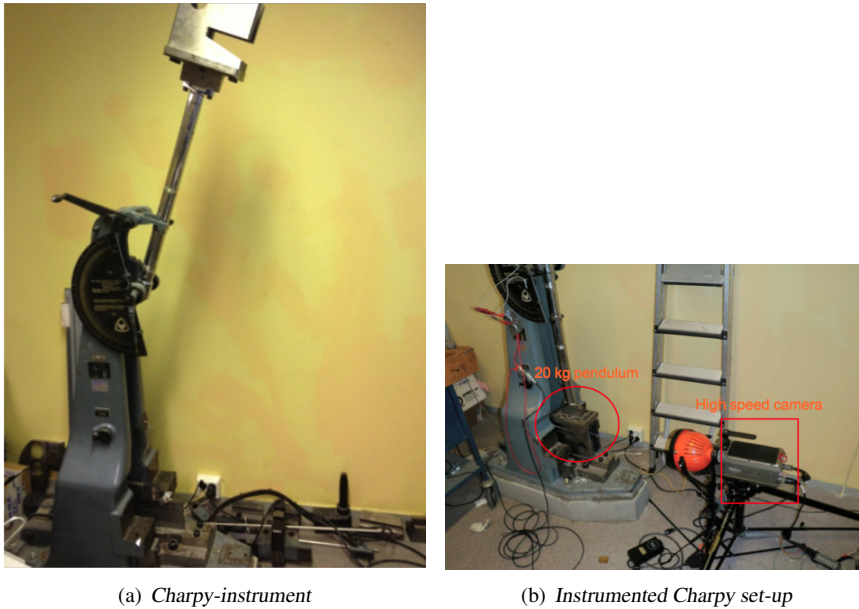
Figure 4.3: Charpy machine and test set-up used during testing [93, 94].
